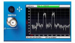
The LCD display and its associated joystick is used for configuration and monitoring.
